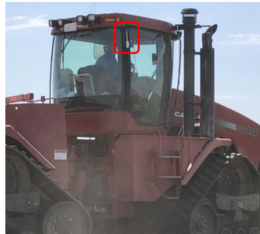
SEEDMASTER AP INSTALLED ON TRACTOR CABS BACK MOUNTING BAR
