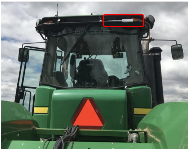
SEEDMASTER AP INSTALLED ON TRACTOR CABS BACK MOUNTING BAR
