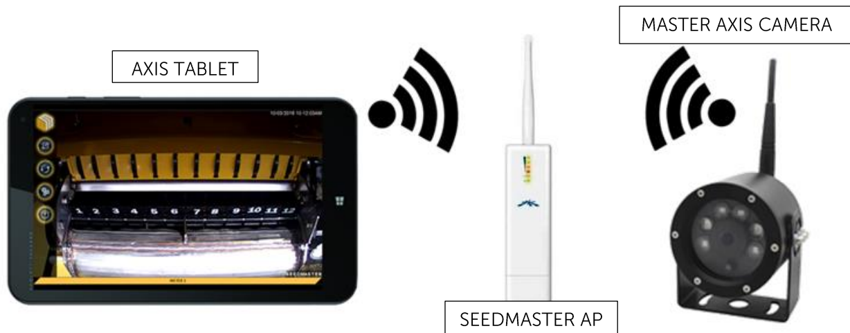
SEEDMASTER AXIS COMPONENTS CONNECTIVITY DRAWING
